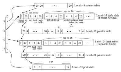
Fig. 3 Data structure for the proposed 8-8-8-8 table.
